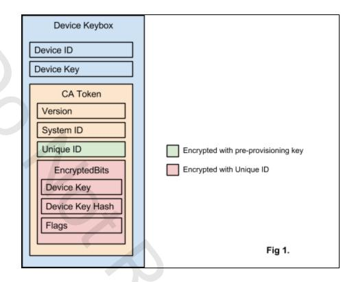
The Device Keybox uses AES-128 keys. Each device is factory provisioned with a device-unique keybox. When a DRM license is needed, the CA Token in Fig. 1 above is sent to the DRM License Server to authenticate the device.
