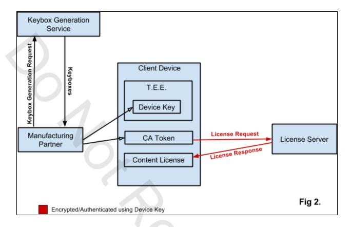
The above diagram shows the provisioning and application of device keyboxes in Provisioning 1.0
