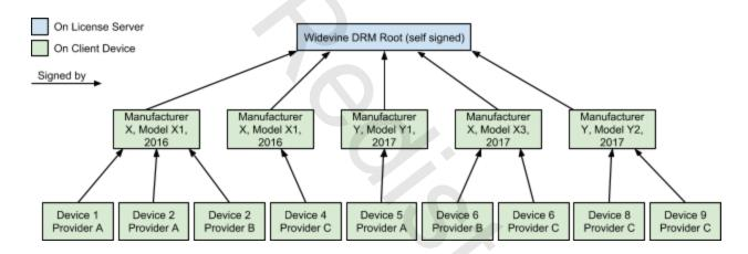
Each device may have a number of device DRM certificates, one for each content provider it has accessed. Each of these is signed by a common intermediate make / model type certificate, which in turn is signed by the Widevine DRM root certificate. The unit of revocation in this case is the device make / model. Revocation is performed by revoking the intermediate make / model type certificate.
