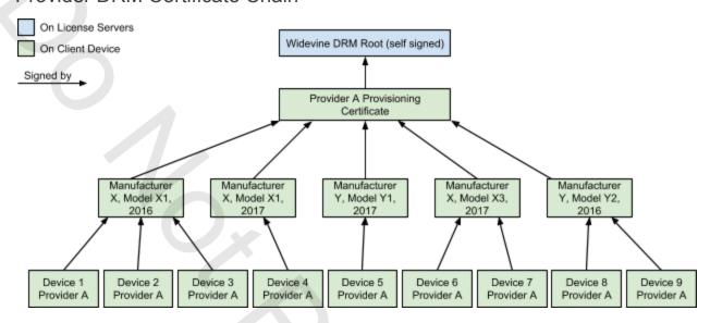
In this scenario, the Provider requests a Provisioning Certificate from Widevine. It can then use this certificate to generate intermediate device certificates for any device types registered with Widevine, as well as DRM device certificates for use with its license server. These DRM device certificates are not valid for use with any other provider's services.
